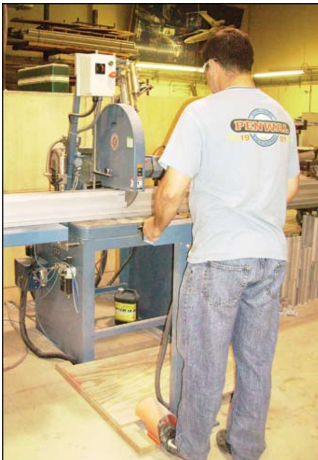
Cutting the aluminum extrusions to order is simple and quick. Here the framing members are done at Penwal Industries, Rancho Cucamonga, CA, under contract to Kithaus, one of two MHS licensees in California.
